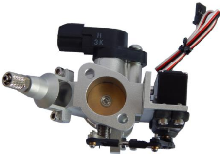
Throttle body with TPS and Servo motor
